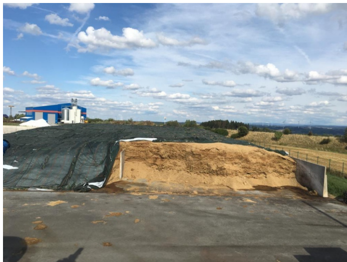
Picture 3: Feedstock storage yard model storing press mud for 6 months during off season
